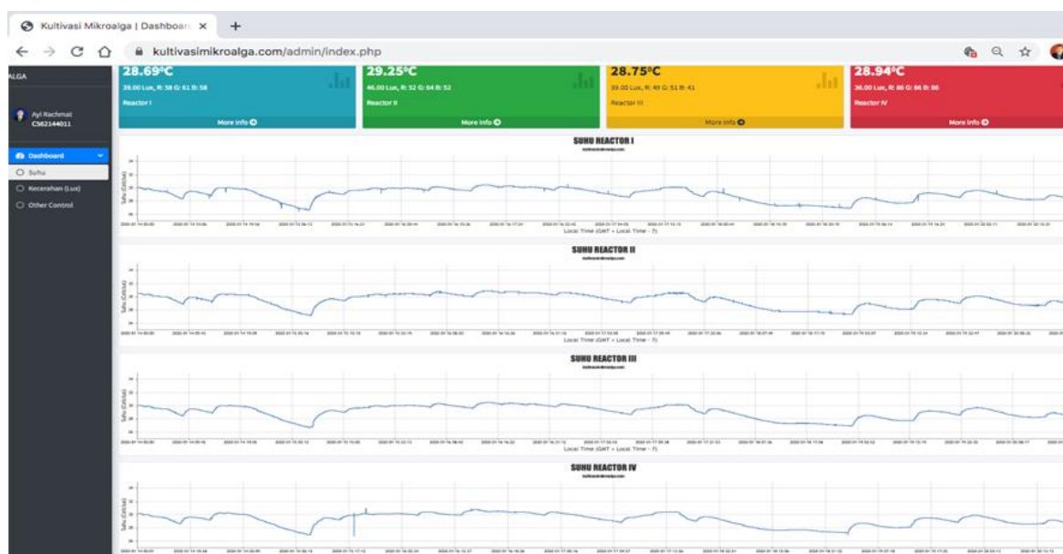
Figure 7. Display from the web https://kultivasimikroalga.com/admin/index.php on a graph display temperature monitored continuously at a set point 30 °C
